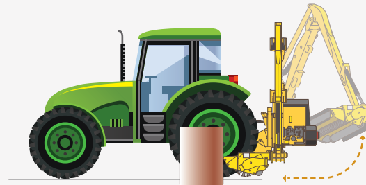
Hydraulic safety breakaway enables the Power Arm to break backwards and upwards on contact with an obstacle
