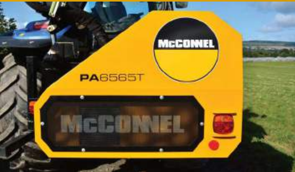
Integrated Oil Cooler
