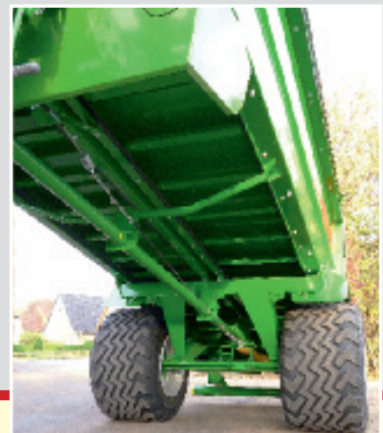
The full-steel bin without base frame saves weight and facilitates cleaning of the spreader.
