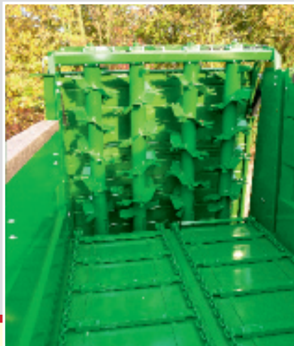
Solid scraper floor bars bolted close together guarantee an optimal supply of the material to the beaters.
