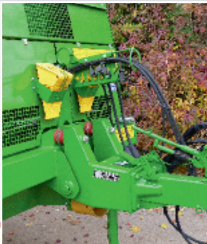
Overrun device with automatic reverse in connection with sprung drawbar. Unique in this class!
