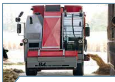
Cross conveyor at the front with side shift (optional)
