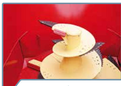
Foreign object magnets on the mixing auger
