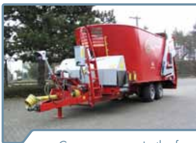
Cross conveyor in the front
