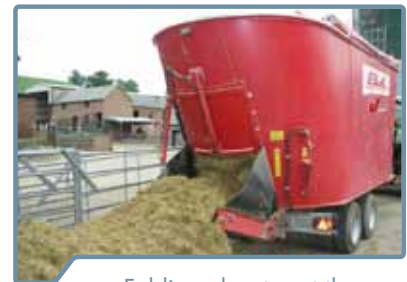
Folding elevator at the rear
