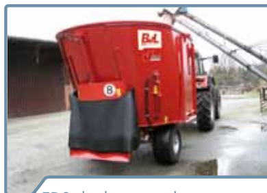
EDS discharge at the center rear
