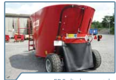
EDS discharge at the center rear
