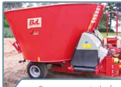
Cross conveyor in the front
