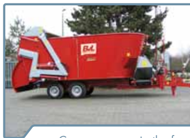
Cross conveyor in the front
