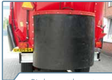
Discharge at the center rear
