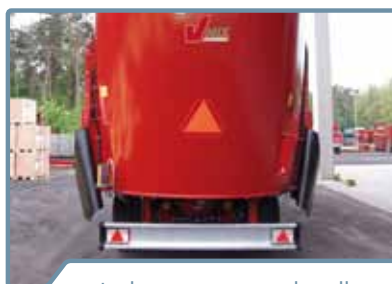
Lighting system with collision protection device
