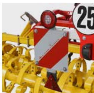
Warning signs and lighting
