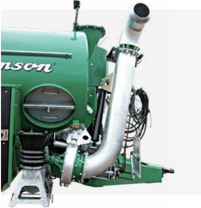
SAP 1* Single link side-mounted filling arm with integrated pump. Simple and fast filling of the slurry tanker from a low funnel.
