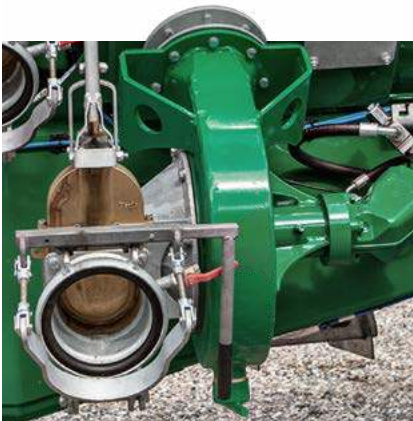
Side-mounted filling pump* Side-mounted filling pump with manual slide valve and quick hose coupling.
