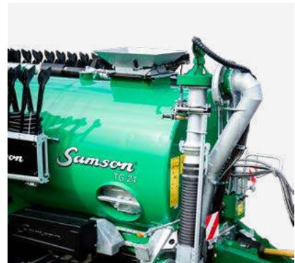
External filling Rear or front mounted wide filling funnel for external filling. The funnel can be opened via a hydraulic slide valve to allow external filling from a stationary or mobile pump unit.
