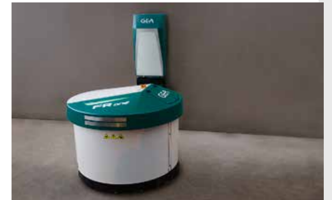
The FRone returns to its charging station automatically and can leave the station either forwards or backwards.
