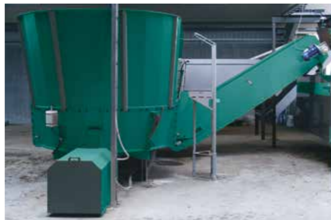
Minimum effort required to fill the stationary feed mixer (volume span 6.5 – 30 m³).
