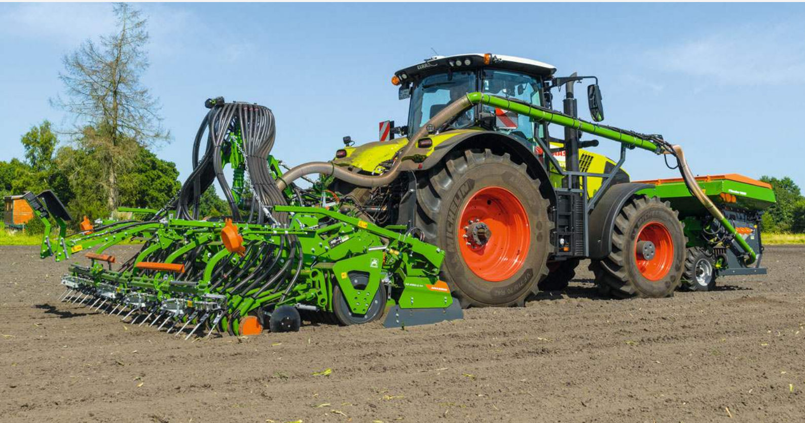
KE 4502-2-300 rotary harrow with Avant 02 seed drill combination and FTender 1600 front-mounted hopper
