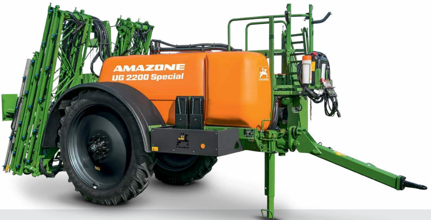
UG 2200 Special with Super-S2 boom in 21 m working width
