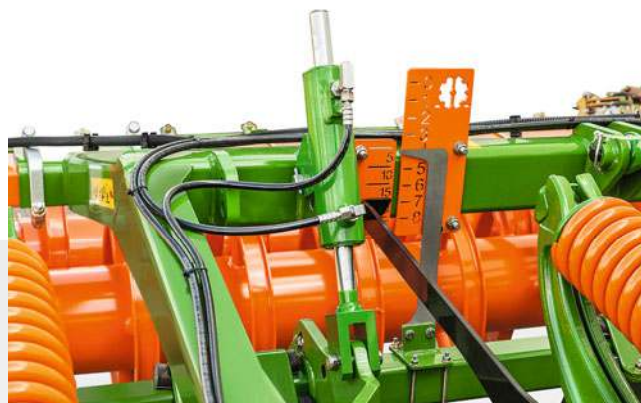
Hydraulic cylinder for setting the depth of the levelling unit
