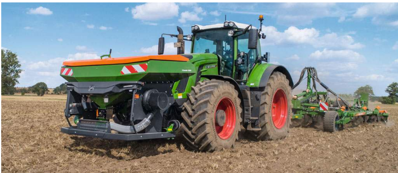
FTender 1600 front-mounted hopper with a capacity of 1,600 l in use with the Cenius 5003-2TX
