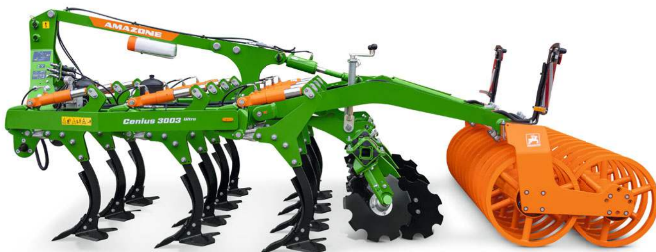
Cenius 3003 Ultra with C-Mix Ultra tines with hydraulic overload protection
