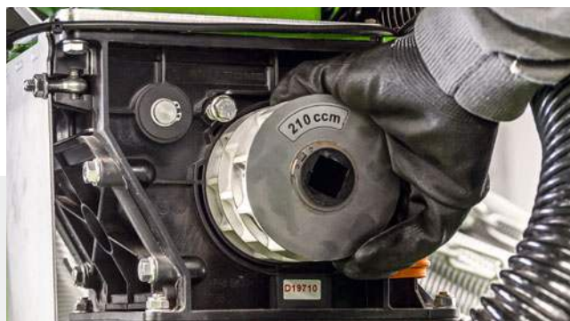
Easy exchange of the metering cassettes
