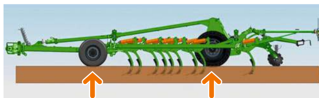
Depth control via support wheels and the running gear
