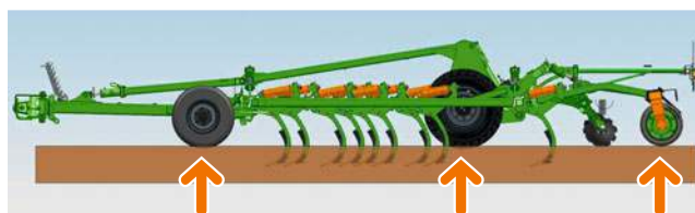
Depth control via support wheels, running gear and the rear roller
