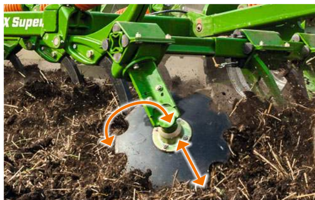
The end discs – individually adjustable in height and angle
