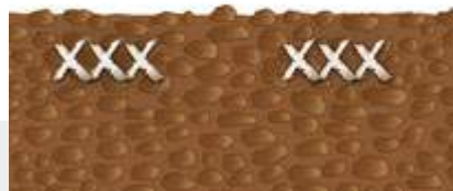
Single-Shoot: 2 or 3 applied materials at one placement depth
