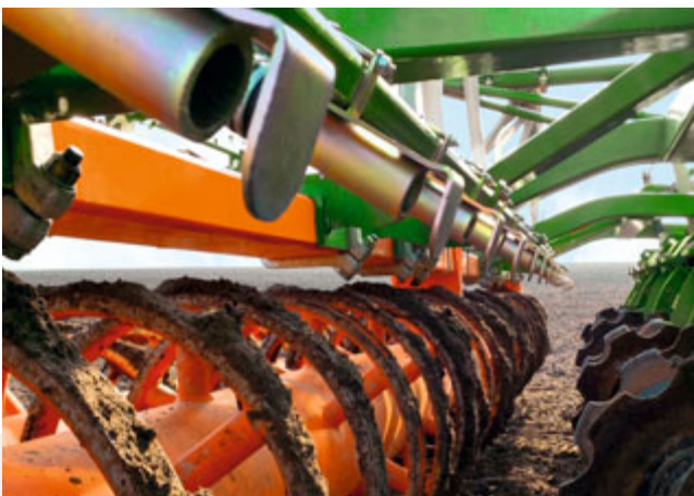
Seed baffle plates for broadcasting on the surface in front of the roller
