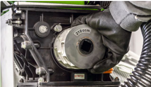
Easy exchange of the metering rollers
