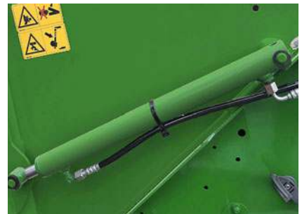
Double-acting hydraulic cylinder
