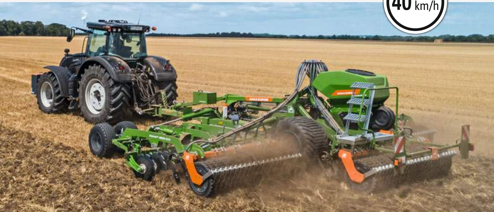
Catros XL 8003-2TX being used for stubble breaking
