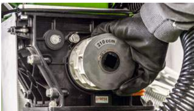
Easy exchange of the metering rollers
