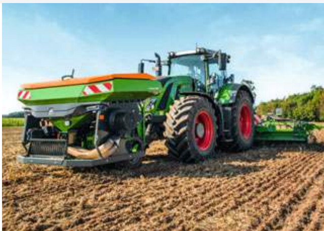
FTender 1600 mounted front hopper with a capacity of 1,600 l
