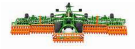
Catros trailed compact disc harrows Working width 7 m to 12 m
