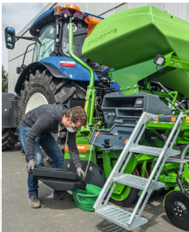
Comfortable emptying of the calibration tray
