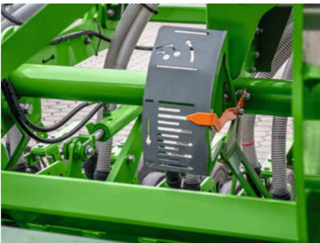
Highly visible scale for coulters pressure adjustment
