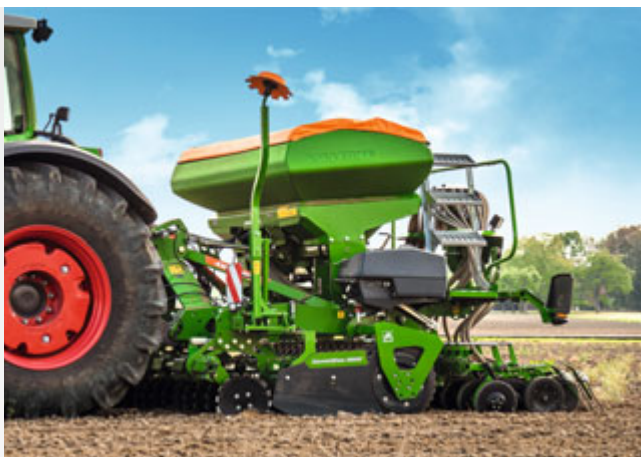
The Centaya 3000 Super harrow-mounted seed drill with CombiDisc 3000 compact disc harrow
