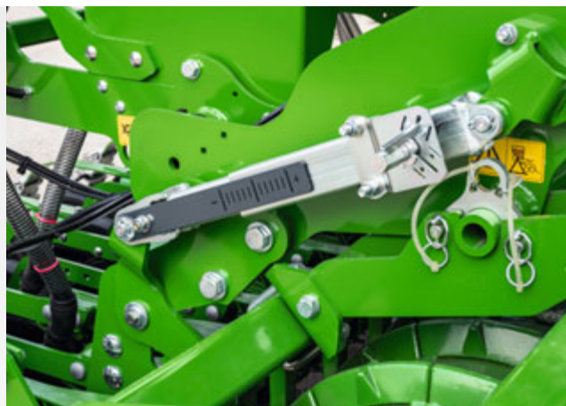
Simple adjustment of the placement depth on the side of the machine
