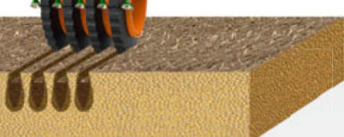
Wedge ring roller with Matrix tyre profile KWM/600 mm
