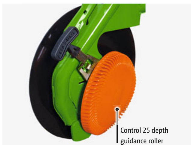
✓ RoTeC coulters (Ø 320 mm) with Control 25 depth guidance roller The cleats, which are open at the rear, provide a very good self-cleaning effect.
