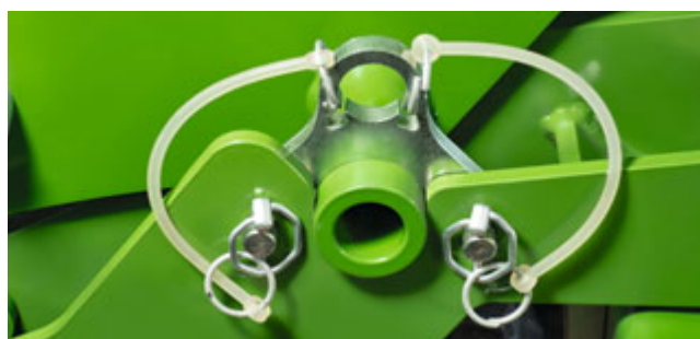
The three easily accessible coupling points of the QuickLink system ensure safe and fast, tool-free coupling and uncoupling.
