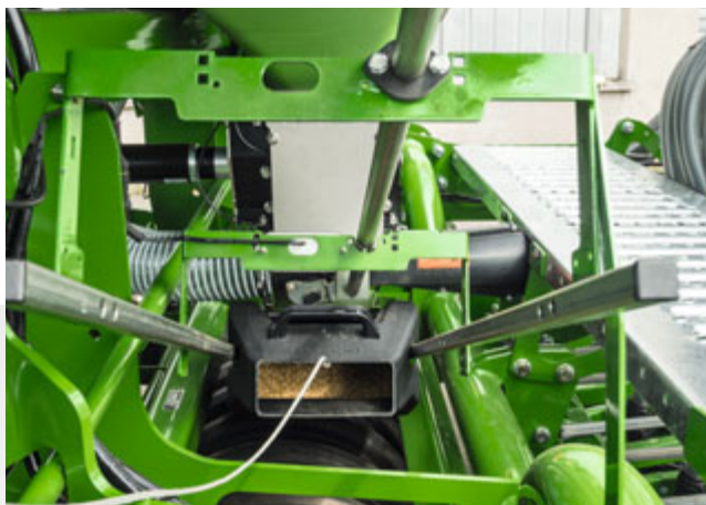
Calibration tray in calibration position
