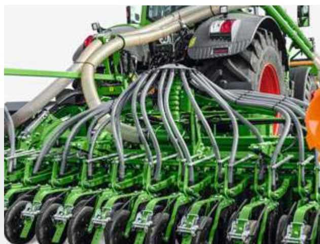
The short seed pipes keep conveying distances to a minimum
