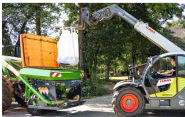
Large opening of 1.10 m x 2.20 m for quick and easy filling of the FTender
