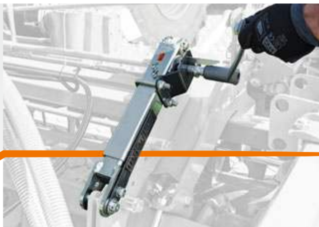
Central adjustment of the sowing depth via the universal setting tool
