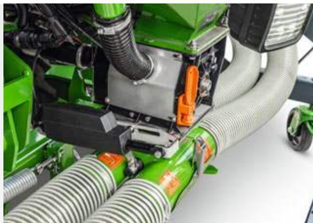
Electric half-side shut-off on the metering unit of the FTender
