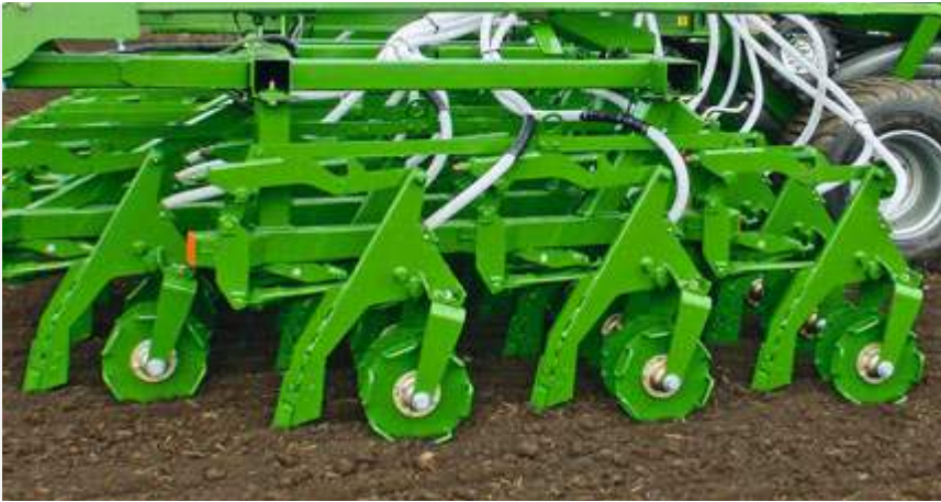
The coulters units are arranged on longitudinal cross members in four rows, which results in a large distance from one to the other. This ensures good straw passage.
