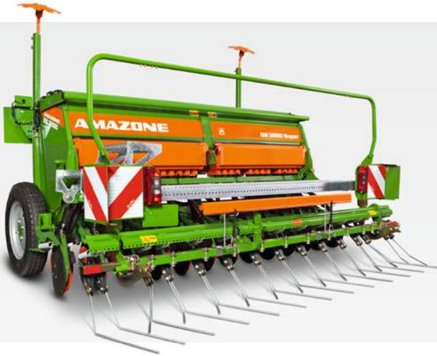
The D9 linkage-mounted seed drill is also ideal for use on its own
